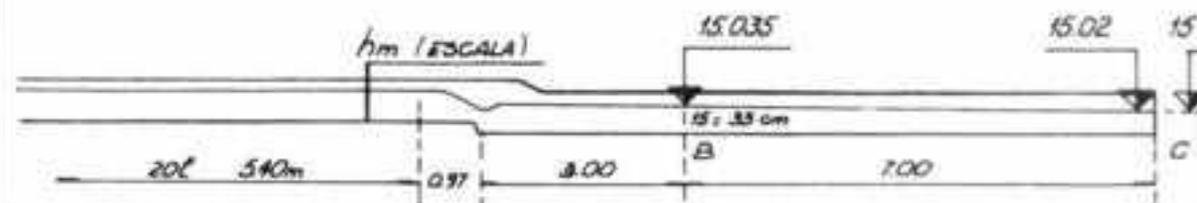
PERDIDA DE CARGA ENTRE LOS PUNTOS B Y C  $W = 0.33 \cdot 0.4 = 0.132 \text{ m}$   $f = 1.00 \text{ m}$
